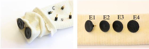
(a) Electrodes placed inside compression bandage. (b) Manufactured electrodes with different surface structures.
