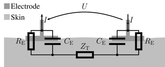
Fig. 1: Equivalent circuit diagram of the passive electrical behavior of electrode-skin contacts.
