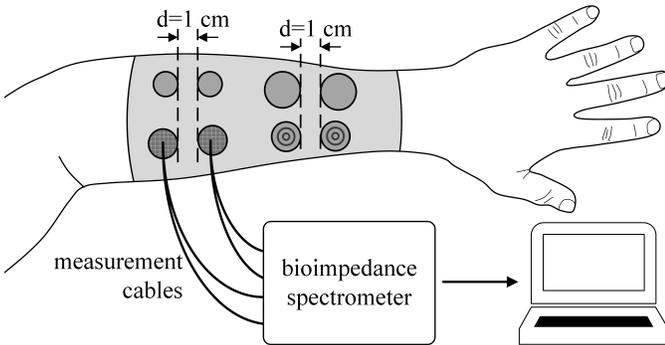
Fig. 4: Measurement setup to determine the electrode-skin interface impedances of different dry electrodes.
