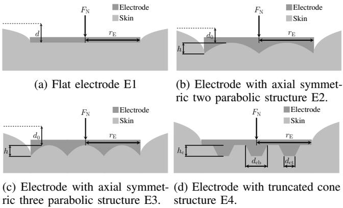
Fig. 2: Electrode cross section.
