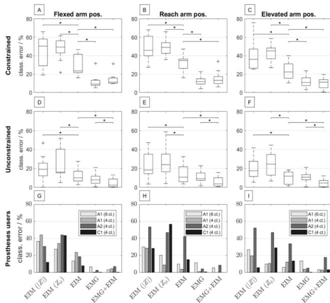
Figure 5. Influence of different combinations of EMG-EIM features, arm positions and muscle contraction types on the classification error when the arm position is not changed between the classifier training and testing. The results are depicted for able-bodied (constrained (A-C), unconstrained (D-F)) and prosthesis users (G-I). A star (\*) denotes statistically significant differences. EMG performs better than EIM, but the combination EMG+EIM can further improve the performance.
