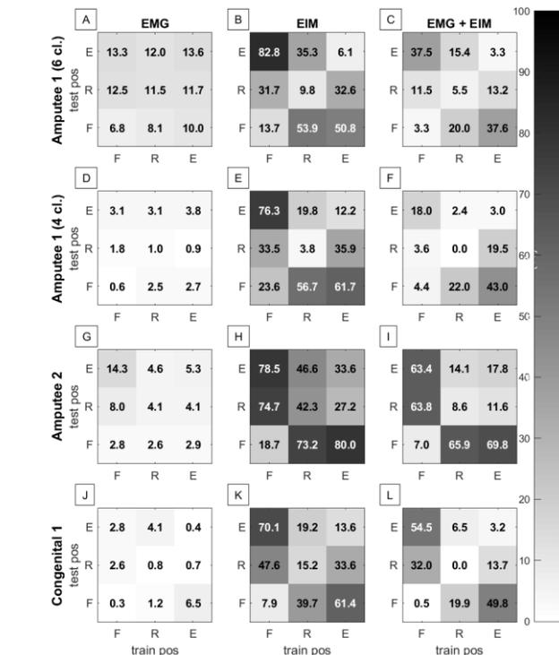
Figure 7. Influence of changing arm position between training and testing on classification error for EMG, EIM, and EMG+EIM classifiers. The depicted classification errors are for individuals with limb deficiency. Annotations F, R, E stand for arm position flexed, reach, and elevated, respectively. Similar to able-bodied, EIM and EMG+EIM are heavily influenced by changing arm position.
