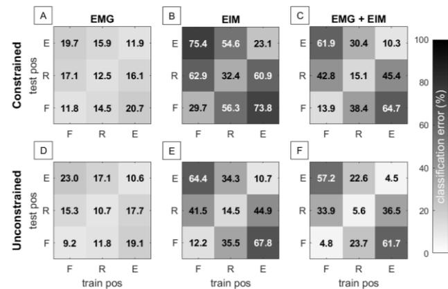
Figure 6. Influence of changing arm position between training and testing on classification error for EMG, EIM and EMG+EIM. The results are depicted for able-bodied subjects in constrained (A-C) and unconstrained (D-F) condition. Annotations F, R, E stand for arm position flexed, reach and elevated, respectively. EIM and EMG+EIM are heavily influenced by changing arm position when trained in one position only.
