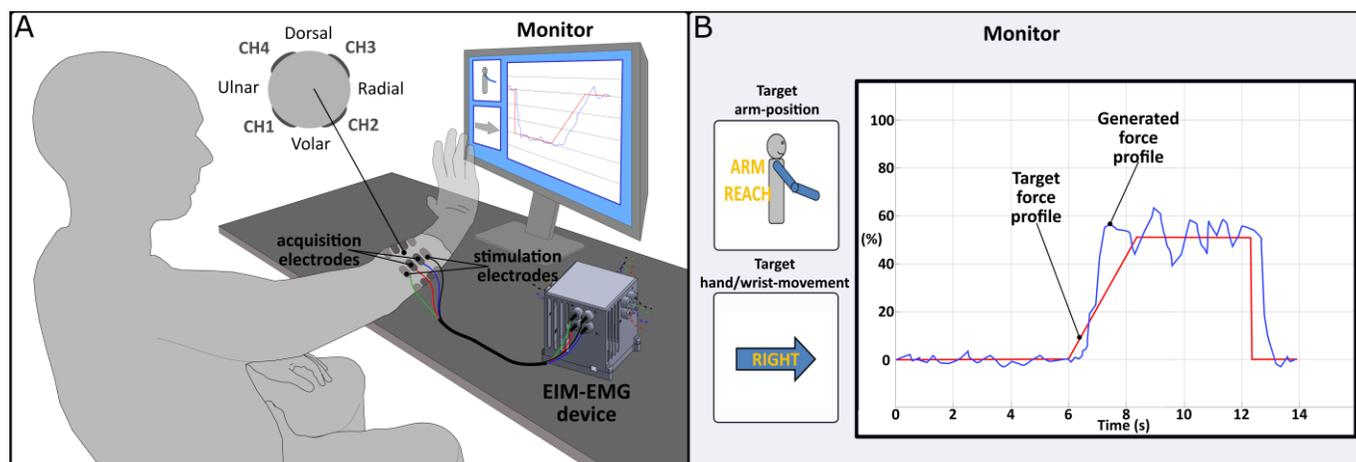
Figure 1. The experimental setup consisted of a device that simultaneously measured EIM and EMG from four recording sites (channels) and a PC for data recording and visual instructions (A). Instructions were provided regarding the arm targeted position, the motion class, and the contraction level. Visual feedback was provided on the contraction level only (B).
