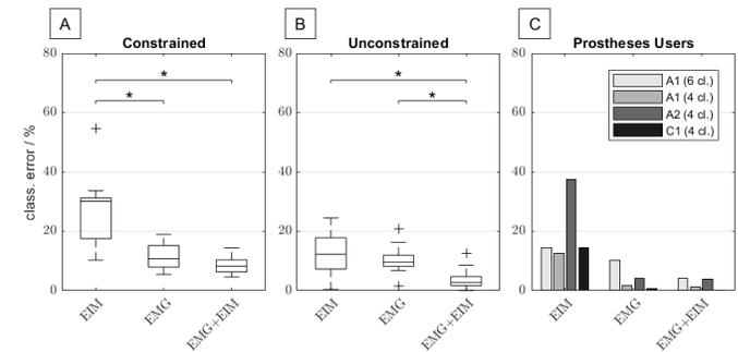
Figure 8. Influence of training with pooled arm position data on the classification error for EMG, EIM and EMG+EIM. The subfigures depict the classification-error of able-bodied participants (constrained (A) and unconstrained (B)) and of prosthesis users (C). A star (\*) denotes statistically significant differences. With the pooled training strategy, the combination of EIM+EMG outperforms EIM or EMG alone in most cases.
