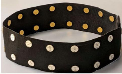
**Figure 2:** Stretchable dry electrodes belt for comfortable and equidistant electrode placement.
