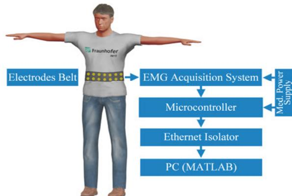
**Figure 1:** Principle of the multi-channel EMG data acquisition from the lower back and abdominal muscles.
