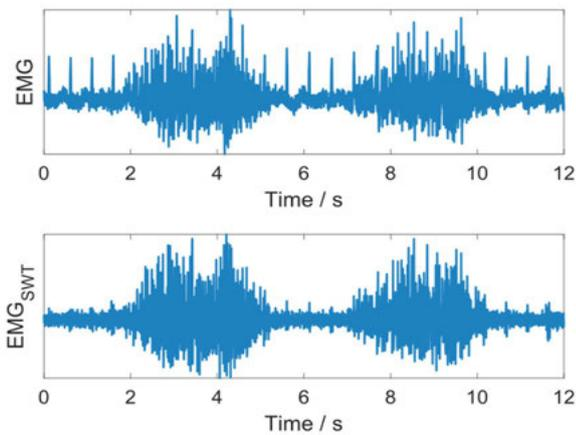
**Figure 5:** Exemplary EMG signal before and after ECG removal via wavelet denoising.
