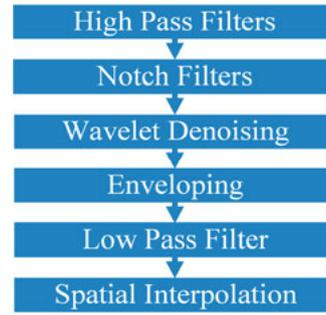
**Figure 4:** Principle of the digital signal processing.
