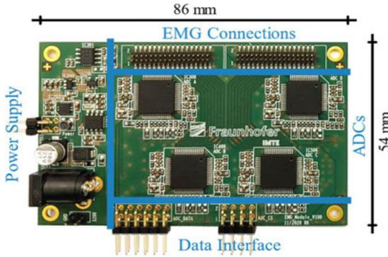
**Figure 3:** Printed circuit board of the EMG acquisition system, capable of digitizing 16 channels, simultaneously.
