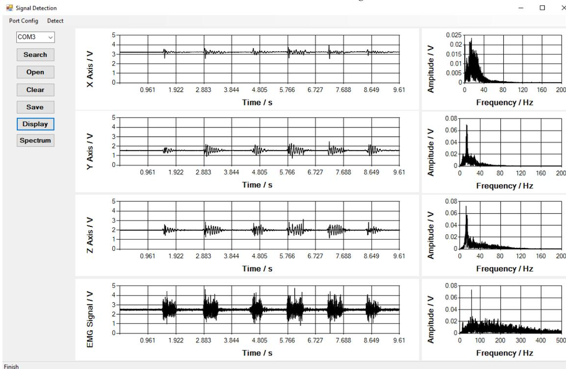
Figure 3: Graphical user interface for data acquisition. The left buttons are function selection, and the middle chart shows the signals collected for a period of time, while the spectrum can be displayed in the four charts on the right after collection.
