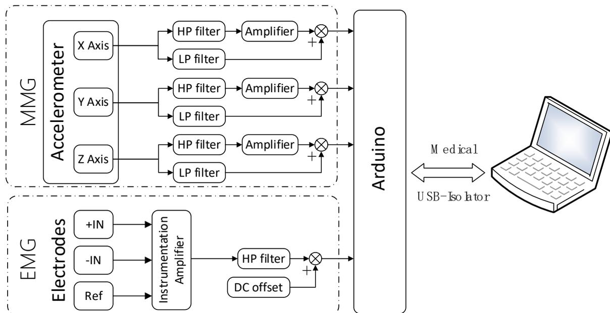
Figure 2: Block diagram of electrical system. (HP = high pass, LP = low pass, Ref = reference, DC = direct current)
