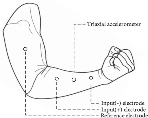
Figure 1: Placement of sensors.
