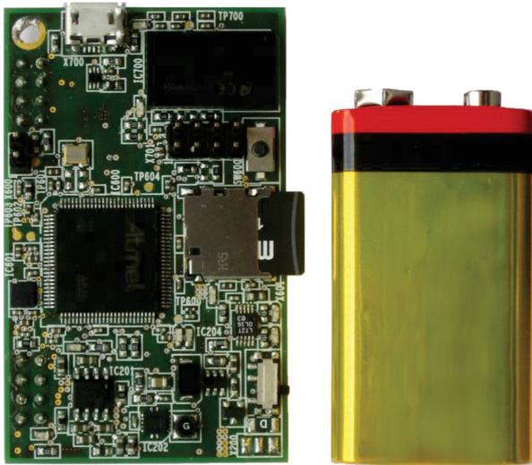
**Figure 5:** Manufactured and populated 6-layer PCB of the measurement system. The PCB contains more than 200 components. The 9 V block battery is shown for comparing the PCB's dimensions.
